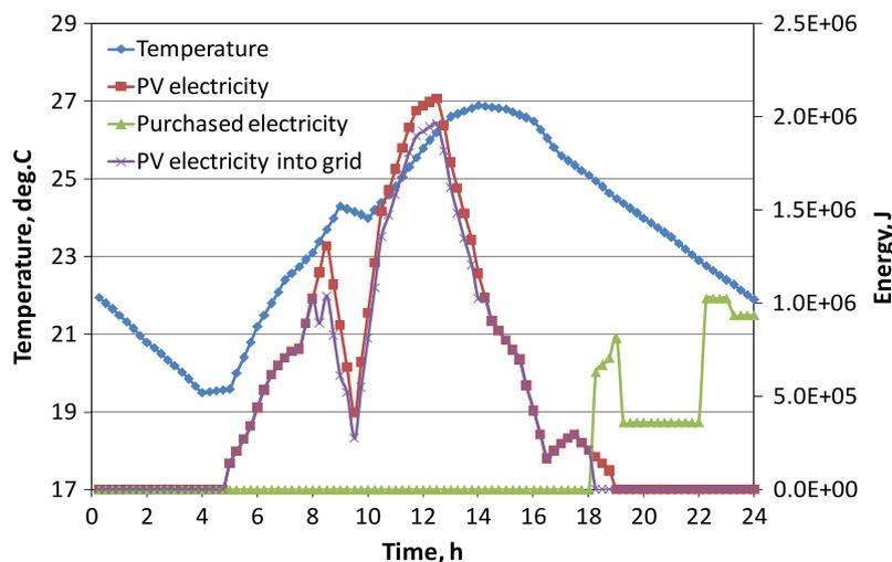
Fig. 6. Different types of electrical energy as a function of time for the third house. Simulation values are given for each 15 min on July 1st.
