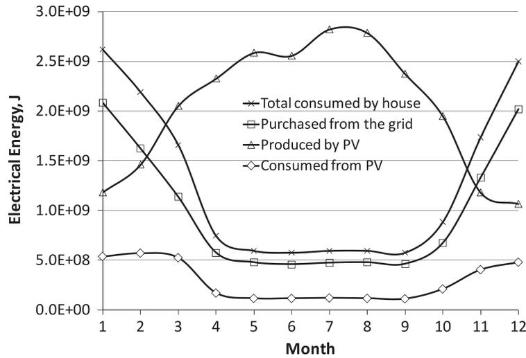
Fig. 7. Monthly values for different types of electrical energy for the third house.
