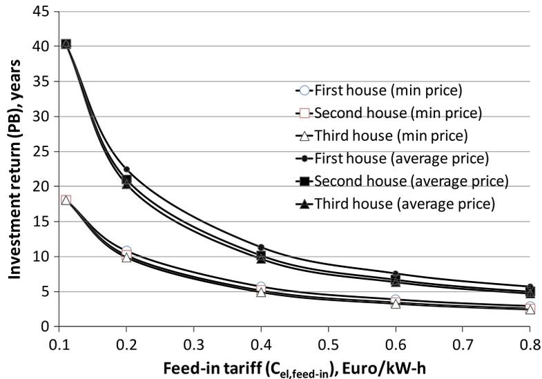
Fig. 12. The investment return of the PV system as a function of the produced electricity selling price.
