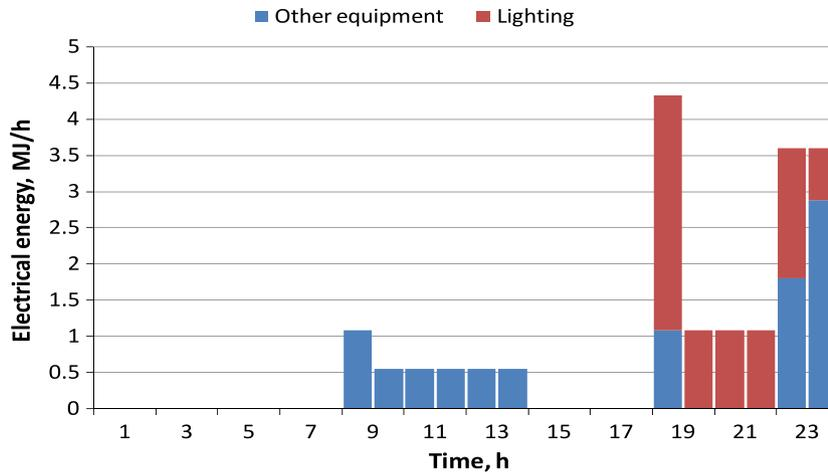
Fig. 4. Electrical energy consumed in the houses for lighting and other equipment (excluding heating): its daily distribution.
