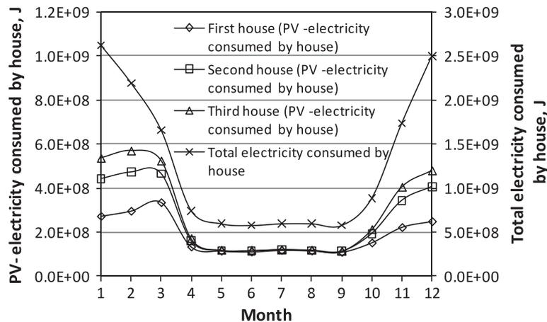
Fig. 9. Monthly values for the electricity consumption directly covered by PV-origin electricity by all three houses. The monthly amounts of the total electrical energy consumed by the houses are also given for comparison.
