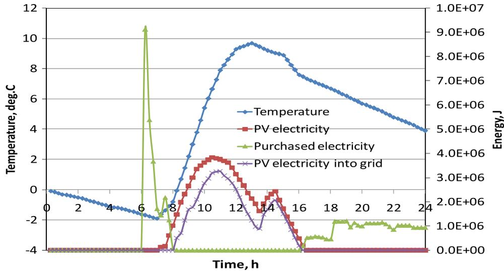
Fig. 5. Different types of electrical energy as a function of time for the third house. Simulation values are given for each 15 min on January 21st.
